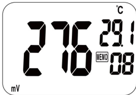
2. Dip the ORP electrode in the sample, stir the ORP electrode gently for about 1 minute, the data can be read and recorded when the value is stable.
